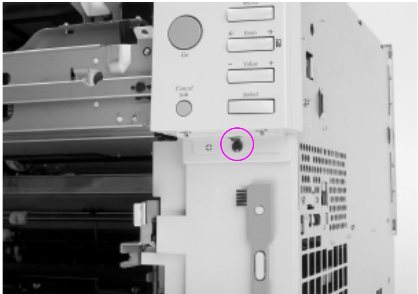
Figure 6-10 Control panel removal and replacement
