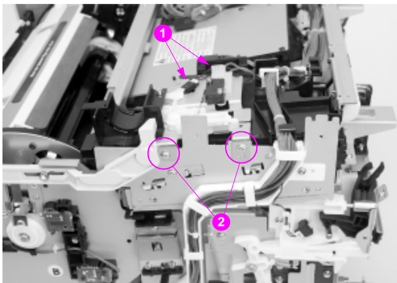
Figure 6-18 Top door switch assembly removal and replacement
