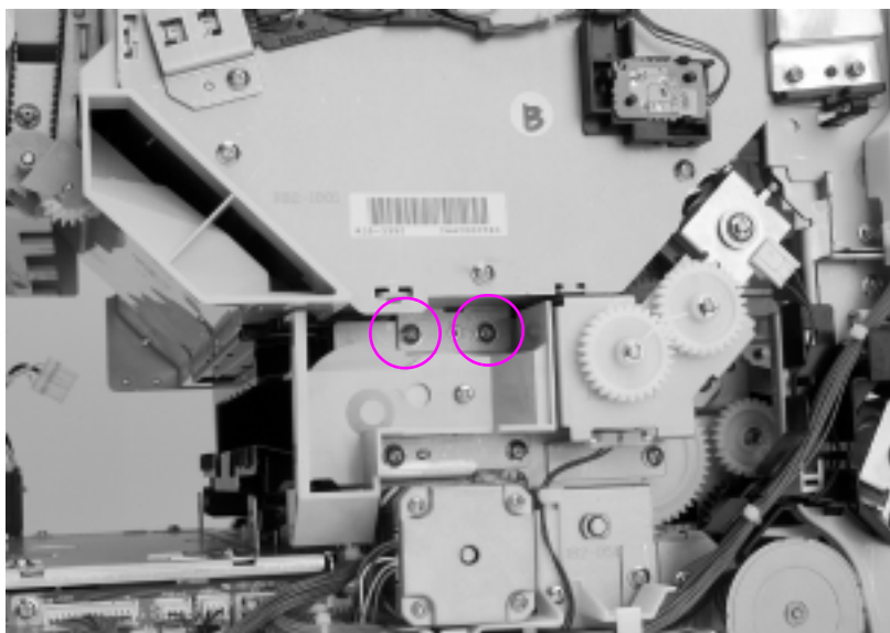
Figure 6-61 Carousel housing assembly removal and replacement (3 of 4)
