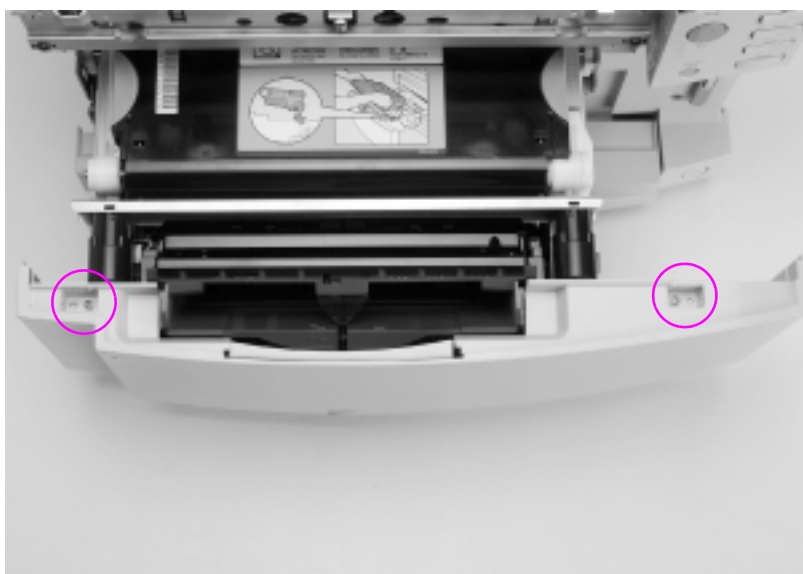
Figure 6-9 Middle front drawer cover removal and replacement
