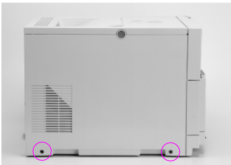
Figure 6-3 Left side cover removal and replacement
